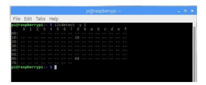
Then, the Program starts scanning and looking at the actually connected I2C devices on Board ET-IOT HAT; **DS2482-100 Address 18** and **DS3231 Address 68**. If the program shows these values, it means that Board ET-IOT HAT is ready to run.
