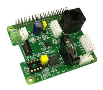
**Board ET-IOT HAT** is particularly designed for using together with Board Raspberry PI by using I2C BUS Interface; so, it can communicate to Board INPUT, OUTPUT or Board SENSORs in the format of I2C BUS Interface or 1-WIRE Interface effectively.
